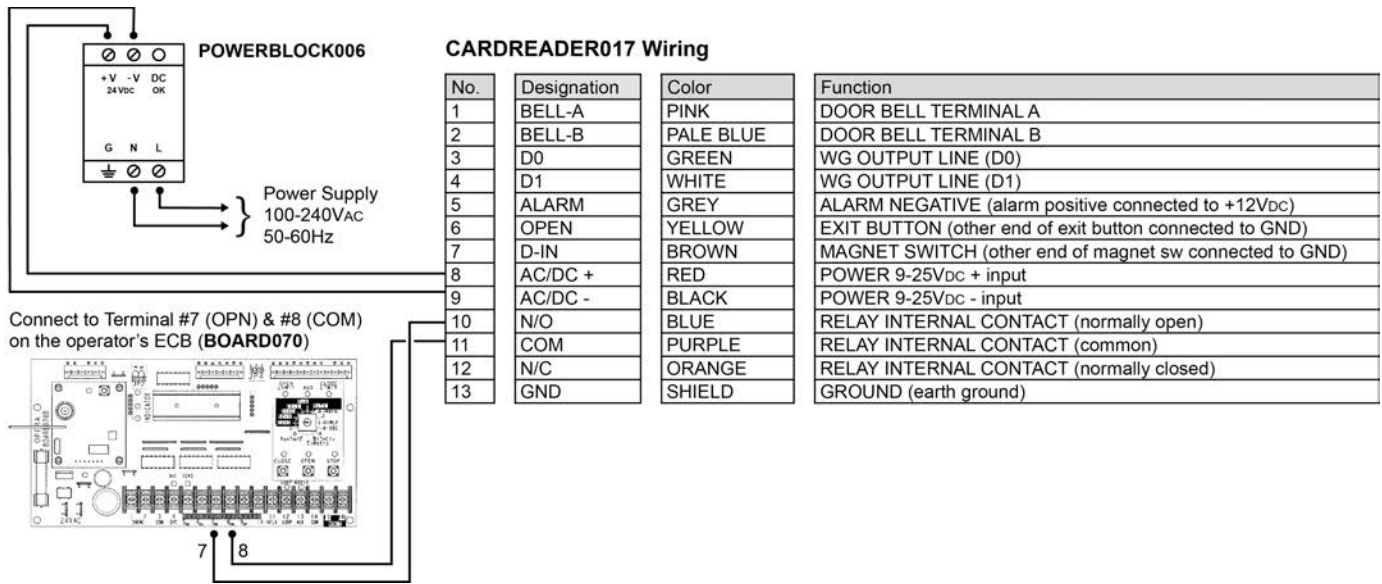
Figure 2 - CARDREADER017 and POWERBLOCK006 Wiring Schematic
