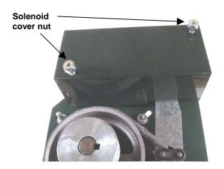
1. Remove the solenoid cover by unscrewing the two nuts.
