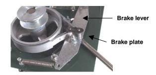
5. Use a screwdriver to press the bottom of the link pins (between the brake plate and brake lever); this will stabilize the pins in their initial position while placing the link.
