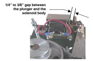
3. The gap between the plunger and the solenoid body should measure 1/4" to 3/8" wide.
