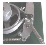
4. Tighten the pivot nut and recheck the gap measurement.
