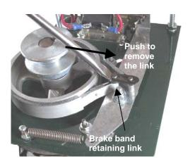
2. Remove the link, which retains both ends of the brake band.
