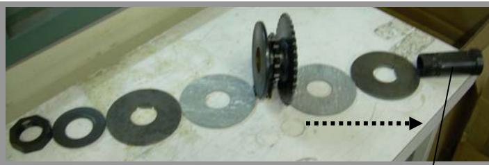
Assembling order on the reducer drive shaft
